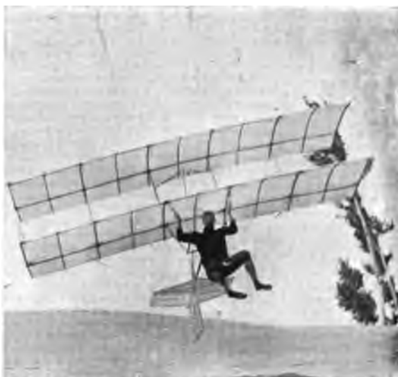
CHANUTE GLIDER STRUCK BY A SIDE GUST; THE BODY SWINGING OVER TO THE RIGHT SIDE (OF THE PHOTOGRAPH) TO RESTORE EQUILIBRIUM
